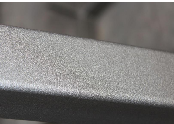
MORN Shot blasting rust removal result
